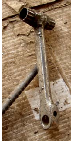
A Hohoe bike mechanic welded a freewheel remover on to an old crank arm, and when it spoiled, welded another one on the other side!
